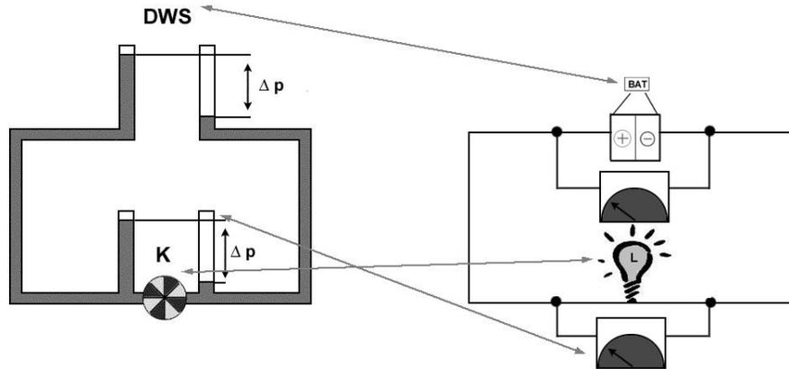
Figure 1: Circuit models of the electrical current analogy
